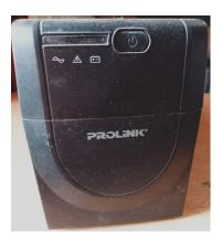
➤ An uninterruptible power supply (UPS) is a device that allows a computer to keep running for at least a short time when incoming power is interrupted. As long as utility power is flowing, it also replenishes and maintains the energy storage.
