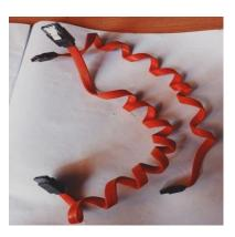
➤ The standard hardware interface for connecting storage and CD/DVD drives to the computer. Introduced in 2001, most computers for consumers use the SATA interface for hard drives.
