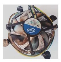
➤ Computer fans are found inside the computer case and help prevent the various computer parts inside from overheating. Without them, components of your computer can malfunction, become damaged, or even crash.
