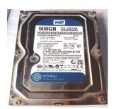
➤ A computer hard disk drive (HDD) is a non-volatile data storage device. Non-volatile refers to storage devices that maintain stored data when turned off. All computers need a storage device, and HDDs are just one example of a type of storage device.
