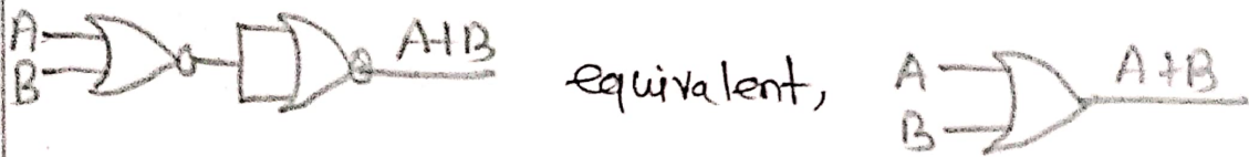
figure: Implementing OR gate using NOR gate
