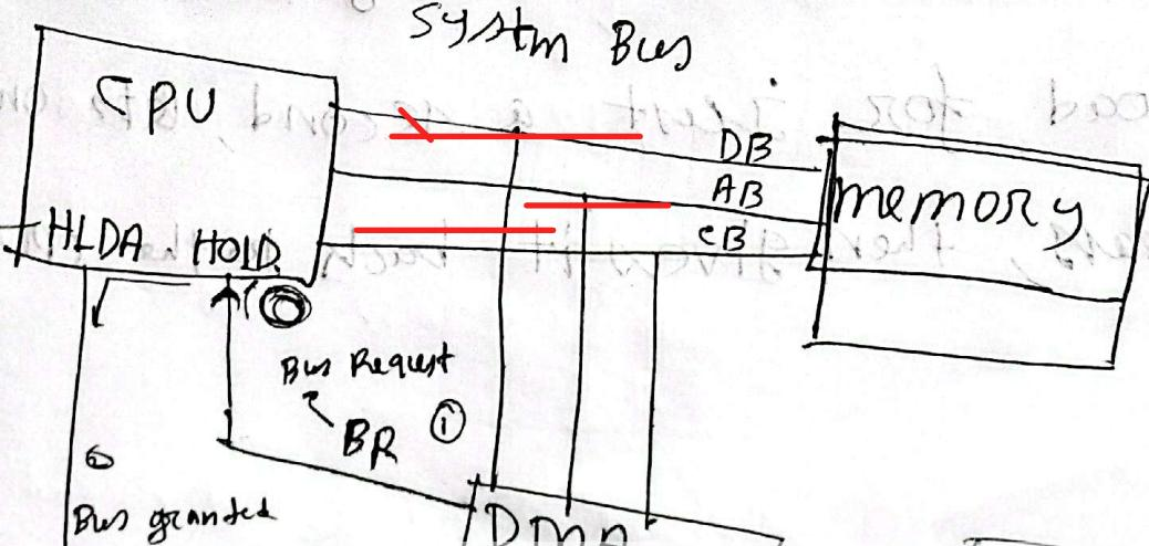
CPU is paused briefly: The CPU stops for a moment so DMA can use the bus to transfer data.
