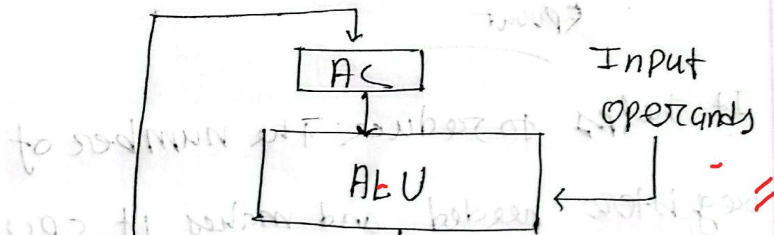
All operations like addition, subtraction, AND, OR, etc are done using the Accumulator and another value from memory
