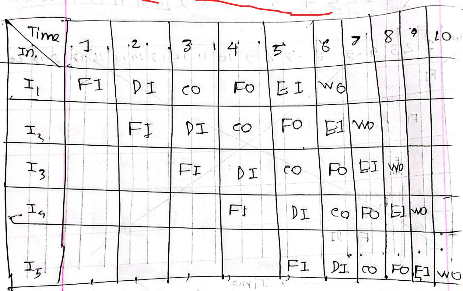
Timing diagram for Pipeline
