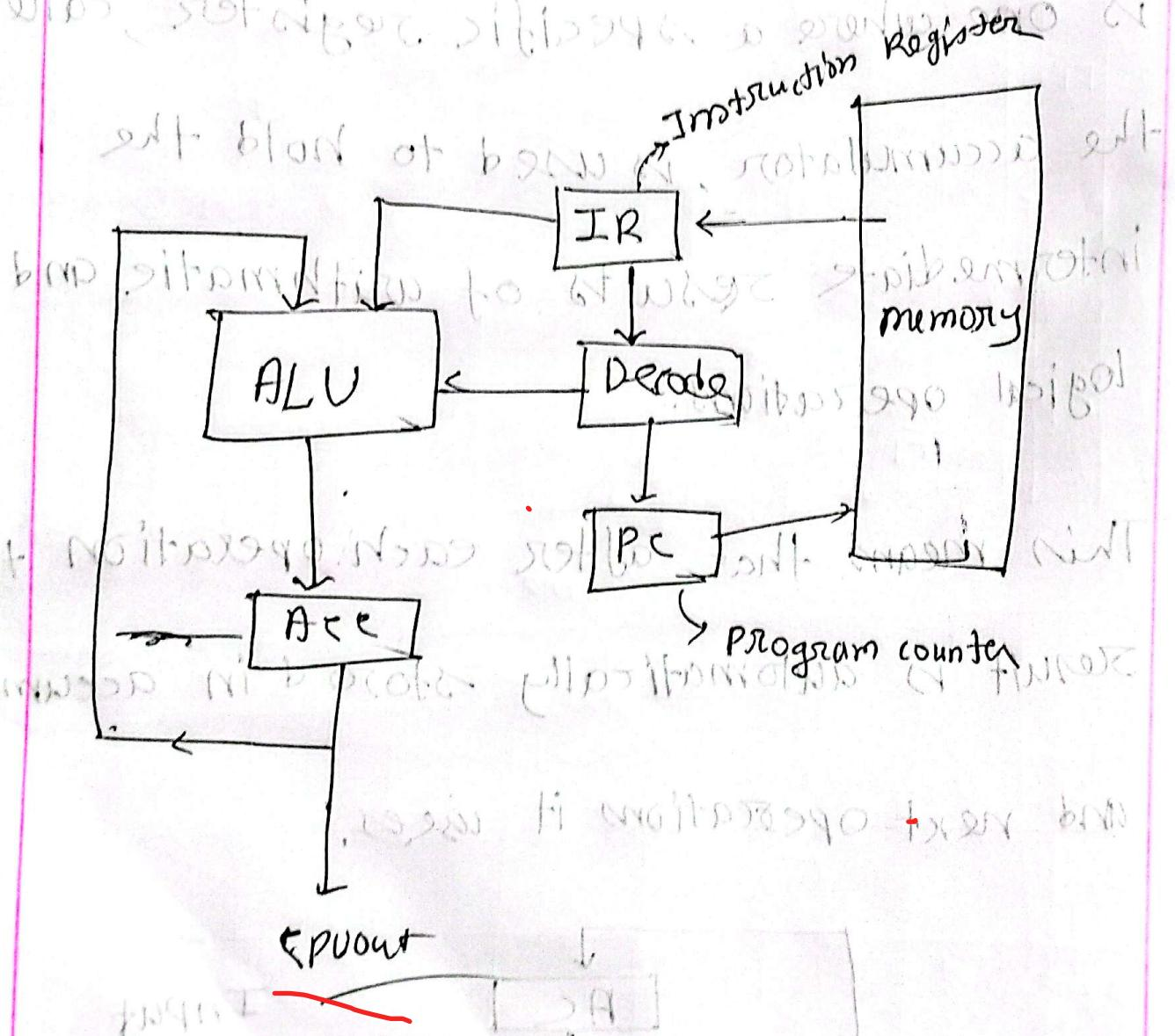
It helps to reduce the number of registers needed, and makes it CPU design simple and faster
