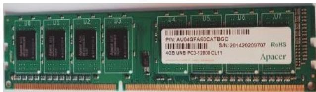
►RAM(Random Access Memory) is an important hardware in a computing device where the operating system, application program and data in current use are kept so they can be quickly reached by the devices processor, It is the main memory of a computer.
