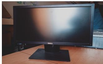
➤ A monitor is known as a screen or a visual display unit (VDU). It is an electronic visual computer display that includes a screen, circuitry and the case in which that circuitry is enclosed.
