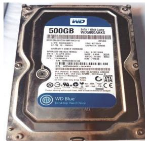
➤ A computer hard disk drive (HDD) is a non-volatile data storage device. Non-volatile refers to storage devices that maintain stored data when turned off. All computers need a storage device, and HDDs are just one example of a type of storage device.
