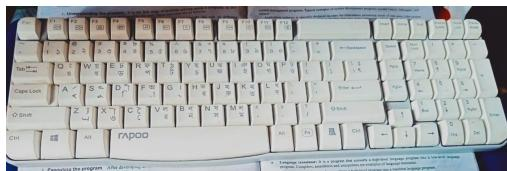
►A computer keyboard is an input device used to enter characters and functions into the computer system by pressing buttons, or keys. It is an important part of a computer system.
