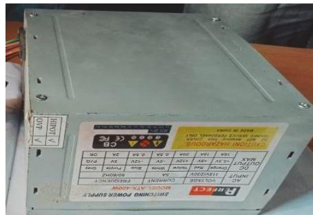
► A power supply is the hardware component that provides electricity to power computers and other devices. It converts electrical current pulled from a power source, such as an outlet, battery or generator, to the correct format and passes it on to a device.
