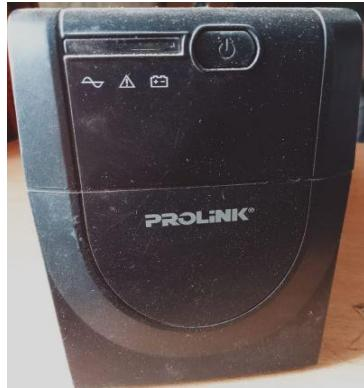
► An uninterruptible power supply (UPS) is a device that allows a computer to keep running for at least a short time when incoming power is interrupted. As long as utility power is flowing, it also replenishes and maintains the energy storage.
