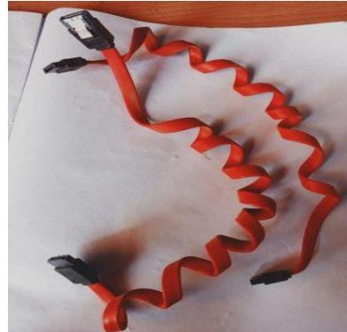
► The standard hardware interface for connecting storage and CD/DVD drives to the computer. Introduced in 2001, most computers for consumers use the SATA interface for hard drives.
