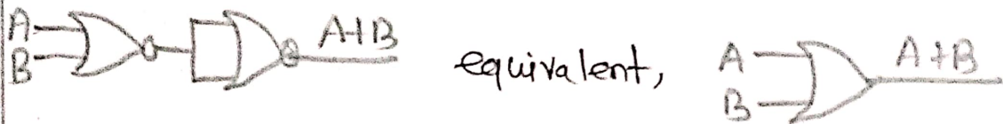
figure: Implementing OR gate using NOR gate
