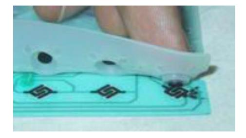
Dome-switches mesh with keys (keyboard is upside down in this image)
