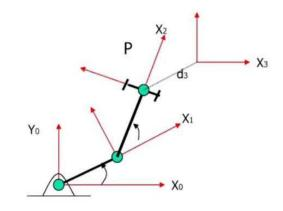
$$T_{base}^{tool} = \begin{bmatrix} C_{123} & -S_{123} & 0 & l_1C_1 + l_2C_{12} \\ S_{123} & C_{123} & 0 & l_1S_1 + l_2S_{12} \\ 0 & 0 & 1 & d_3 \\ 0 & 0 & 0 & 1 \end{bmatrix}$$
