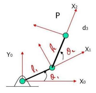
The function atan2 denotes a four quadrant version of arctan function. It allows us to recover angles over the entire range of  $[-\pi \text{ to } \pi]$  if x = y = 0, then the result is indefinite, if x > 0 and y = 0, then atan2 = 0, if x < 0 and y = 0, then atan2 =  $\pi$ , else if y < 0, then  $-\pi < \text{atan2} < 0$ , if y > 0, then  $0 < \text{atan2} < \pi$ .
