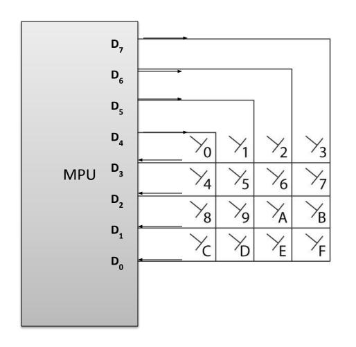
Send Data using Data BUS "D7,D6,D5,D4"
