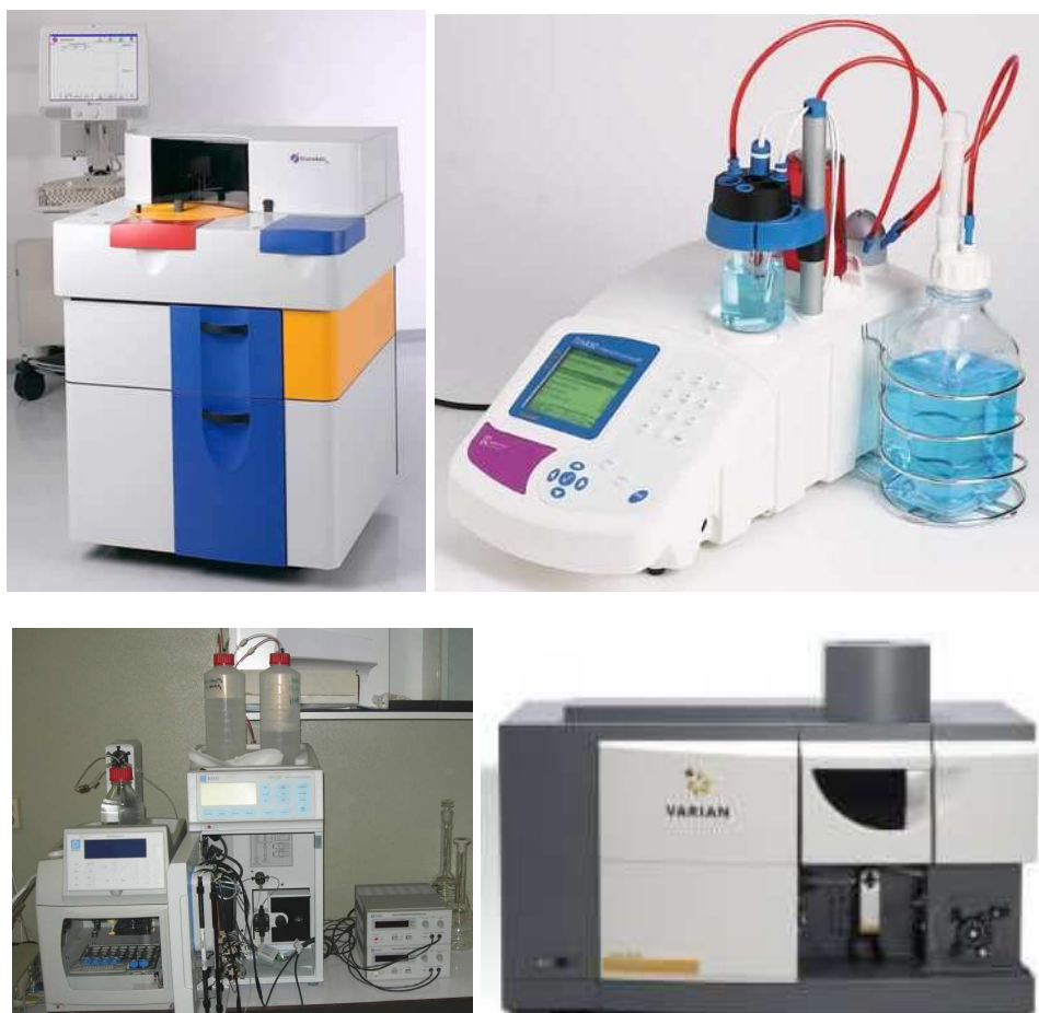
Figure 11.6: Equipment of the VU water laboratory to perform hydrochemical analysis. Aquakem 200 discrete analyser (upper left), Radiometer Titralab TIM840 titration workstation (upper right), Dionex DX-120 IC equipped with IonPac AS14 column (lower left) and Varian 730-ES inductively coupled plasma-optical emission spectroscope (lower right).
