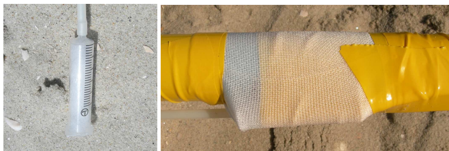
Figure 11.5: A minifilter (right) consists of plastic cylinder (part of syringe) filled with filter wool. One end is attached to the sampling tube and the broad end is open. This filter is attached to the exterior of a piezometer, covered with filter cloth and taped in place on both sides at the desired depth (right).
