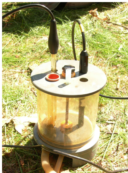
Figure 11.1: PVC–perspex flow through cell with electrodes to measure the pH and EC of water pumped from a well and passing through the cell without being exposed to air.
