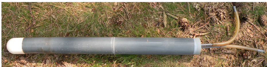
Figure 11.2: Soil moisture suction cup used for the extraction of moisture from the unsaturated zone.
