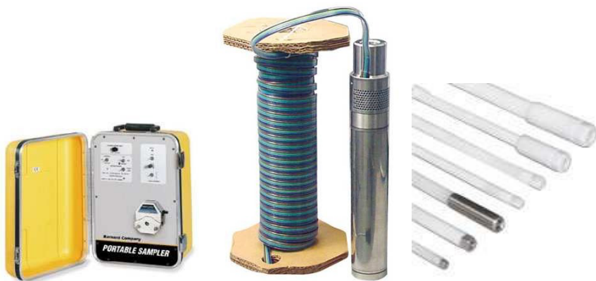
Figure 11.4: Overview of pumps available to collect groundwater: Barnant Company E/S portable water sampler with a peristaltic pump (left), Grundfos submersible pump (center) and Waterra inertial pumps with ball valves (right).
