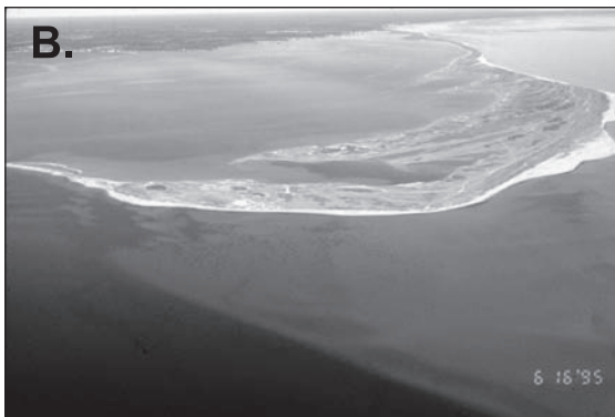
Figure 10.24 Examples of sandy spit development: (A) Map of Buctouche Spit, New Brunswick, Canada; (B) oblique aerial photograph of Buctouche Spit, The spit is about 14 km long from the downdrift end to the point of attachment near the top of the photo. The extensive shoals of the spit platform are evident at the downdrift end. The main tidal channel of the constricted entrance to Buctouche Bay can be seen at the lower left; (C) oblique aerial photo of the distal end of Long Point, Lake Erie. The progradational portion of the spit is about 10 km long.
