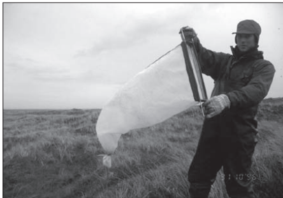
Figure 7.14 Photograph of a streamer trap. The fine mesh bag is attached to a rectangular frame which keeps it open. Several of these are fixed to a vertical post for deployment in the water.
