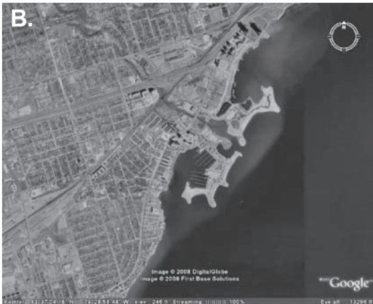
Figure 8.15 (A) Evolution of a log spiral beach down-drift from a seawall on the Illinois shoreline of Lake Michigan (after Terpstra and Chrzatowski, 1992); (B) artificial headlands and crenulate bays on a complex landfill feature, Toronto waterfront, Ontario, Canada; (C) ground view of the armourstone structures forming one of the headland structures in (B) with the Toronto skyline in the background.
