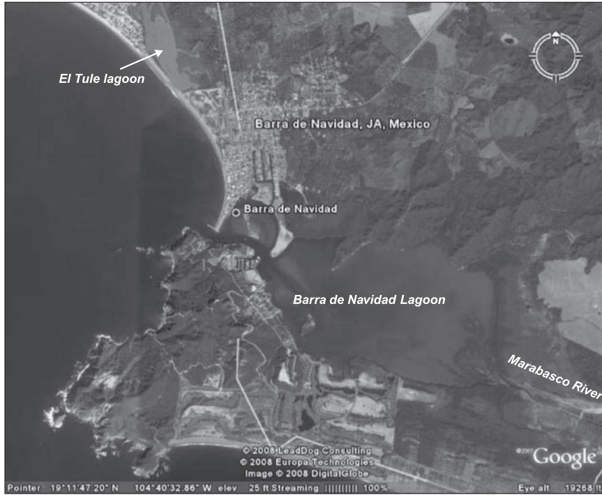
Figure 10.22 Portion of a Landsat image of Jalisco, Mexico showing the Barra de Navidad lagoon and surrounding area. The delta of the Marabasco River has expanded rapidly as a result of increased sediment input from the surrounding hills. The El Tule lagoon near the top left of the picture is an example of a choked lagoon that is only open seasonally during the wet season.
