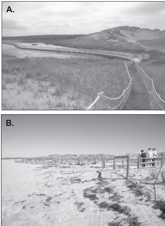
Figure 9.33 Managing people in natural dune areas: (A) nature trail and beach access, Greenwich Dunes, Prince Edward Island National Park. The trail uses a boardwalk to cross stabilised transgressive dunes (background) and the pond in the middle area. The passage across the foredune (foreground) uses a simple set of wooden posts with ropes which act both to keep people to the path and as a handhold up the steep lee slope. A simple plastic mesh on the ground allows some vegetation growth and can be raised to allow sand to fall through; (B) protection of the vegetated embryo dune zone at the back of a beach in NSW, Australia. The fencing is designed as an indication of the protected area, not as a true deterrent to entry, and the open mesh allows natural throughflow of aeolian sand transport.
