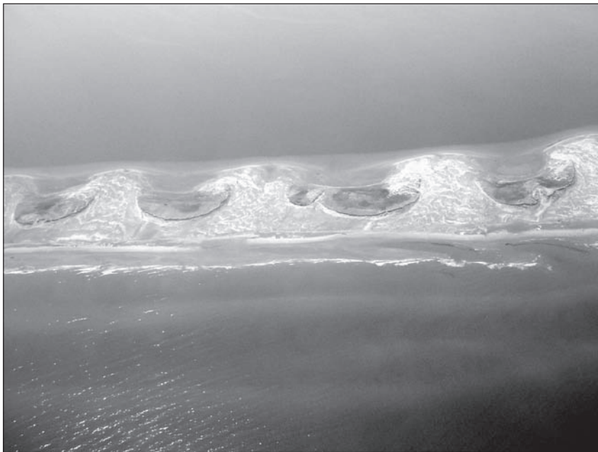
Figure 10.8 Extensive overwash, Cavendish Spit, Prince Edward Island generated by a storm on 28 December 2004. The spatial pattern of overtopping and erosion appears to reflect the alongshore spacing of rip cell/giant cusps with the dune remaining intact opposite the locations with a wider beach.
