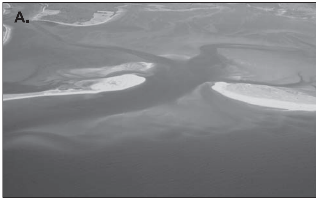
Figure 10.16 Tidal inlets: (A) Little Gulley inlet separating the North and South Kouchibouguac barrier islands (see Figure 10.4). The inlet location is highly stable because of its location opposite the drowned estuary; (B) North Rustico inlet on the north shore of Prince Edward Island. Like many of the small inlets through barriers on the shorelines of the Gulf of St. Lawrence the inlet entrance is stabilised by jetties to protect small harbours for fishing boats; (C) North Inlet, a temporary inlet through the North Kouchibouguac barrier which was breached in 1970 and closed by 1976.
