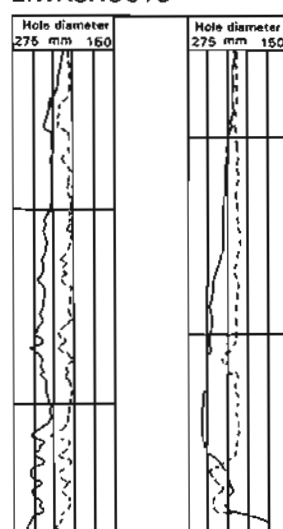
Figure 4.10 Field examples of hole size enlargement seen on the two-arm, dual caliper. 1. Breakouts, seen as well-defined, oval hole developments. 2. Washouts, seen as generalised hole ovality. Hole diameter increases to the left (from Cox, 1983).
