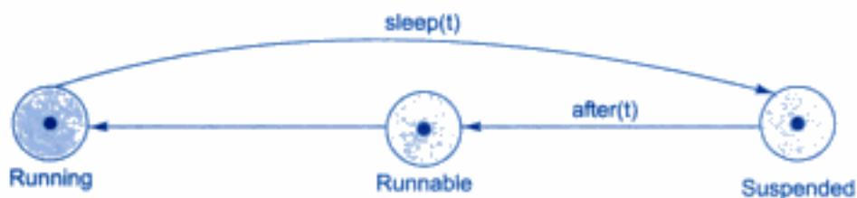
Fig. 12.7 Relinquishing control using sleep() method
