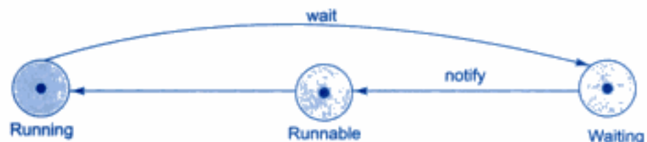
Fig. 12.8 Relinquishing control using wait() method
