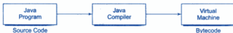
Fig. 3.6 Process of compilation
