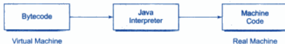
Fig. 3.7 Process of converting bytecode into machine code
