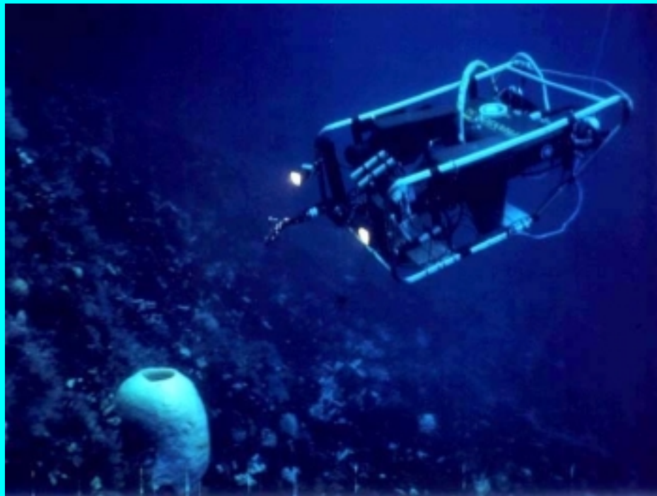
TROV in Antarctica operating under water
